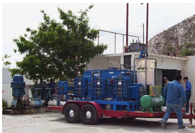
Fig. 7. A picture of the Lamar Mobil Pilot EC Reactor that is being used in Torreón Coahuila México for field trials.
